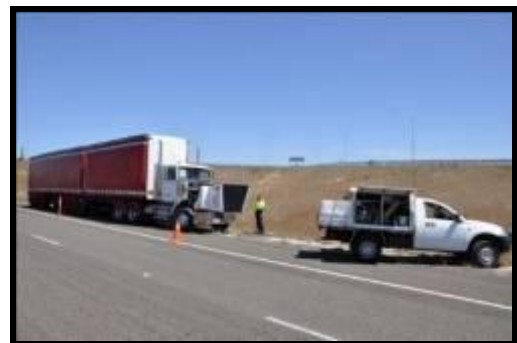
Parking in front of the disabled truck with clearance between truck and service vehicle creates a safe work zone.
