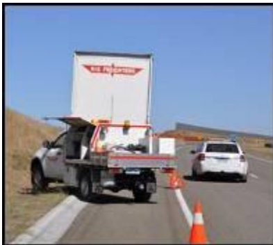
In this position, the mechanic is protected from passing traffic and can safely access both sides of the service vehicle.
