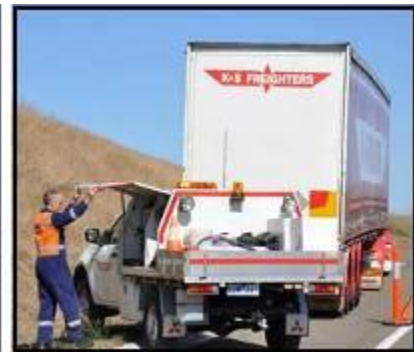
In this position, the mechanic is protected from passing traffic and can safely access both sides of the service vehicle.
