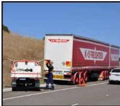
In this position, the mechanic is protected from passing traffic and can safely access both sides of the service vehicle.
