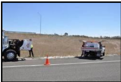
Parking in front of the disabled truck with clearance between truck and service vehicle creates a safe work zone.
