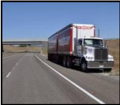
Traffic approaching from behind can't see the truck due to the bridge and curve in the road.
