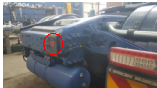
Figure 5: Overview of battery's location in the rear overhang of the prime mover
