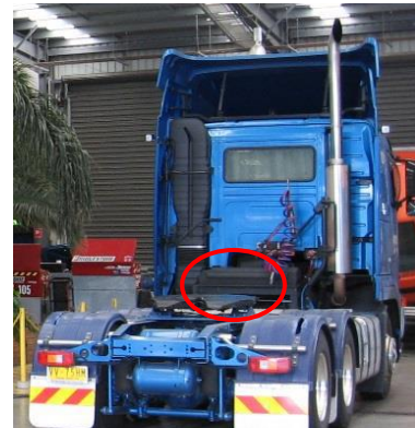
Figure 7: Common battery location on a COE prime mover
