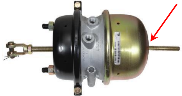
Figure 9: Rated stroke marking location for all spring brake actuator
