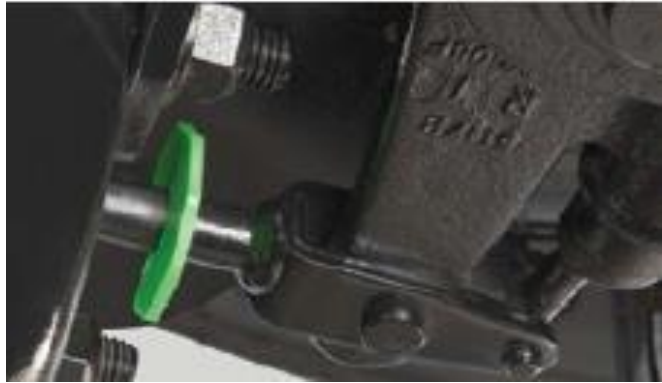
Figure 15: SimpleCheck tool in position on the push-rod of the brake actuator with the brakes applied
