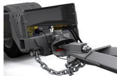
Example of safety chains fitted between the trailer drawbar and truck towbar.
