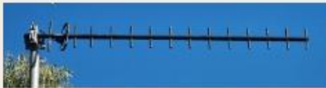
3G Only - Nearly all the elements on the antenna are the same length.
