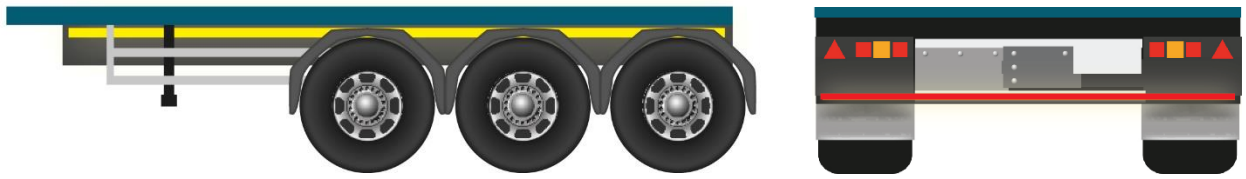
Figure 19: Semi-trailer with tray and line markings
