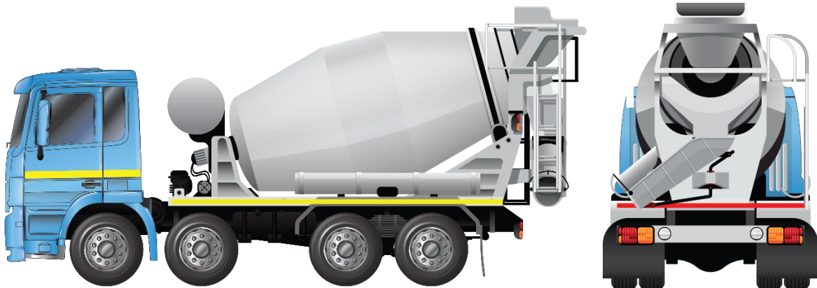
Figure 20: Concrete mixer/agitator with line markings
