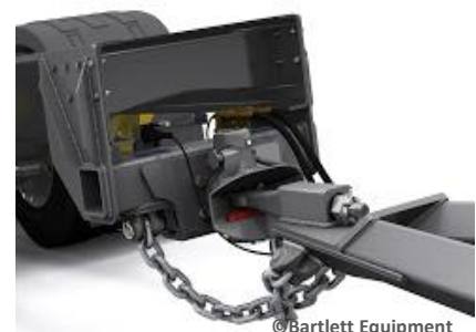
©Bartlett Equipment Example of safety chains fitted between the trailer drawbar and truck towbar. Source: Bartlett Equipment
