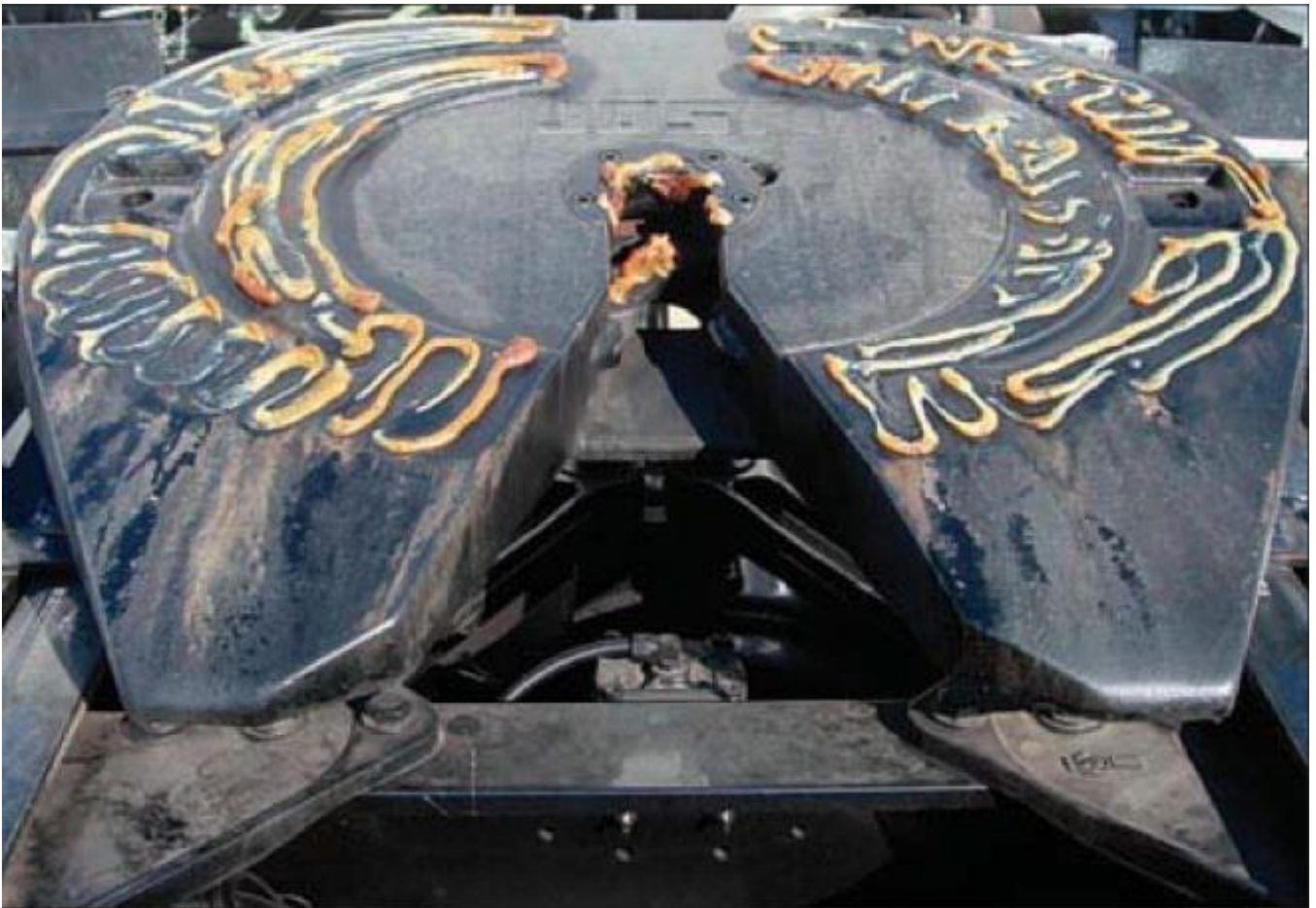
Figure 5: Fifth wheel top plate
