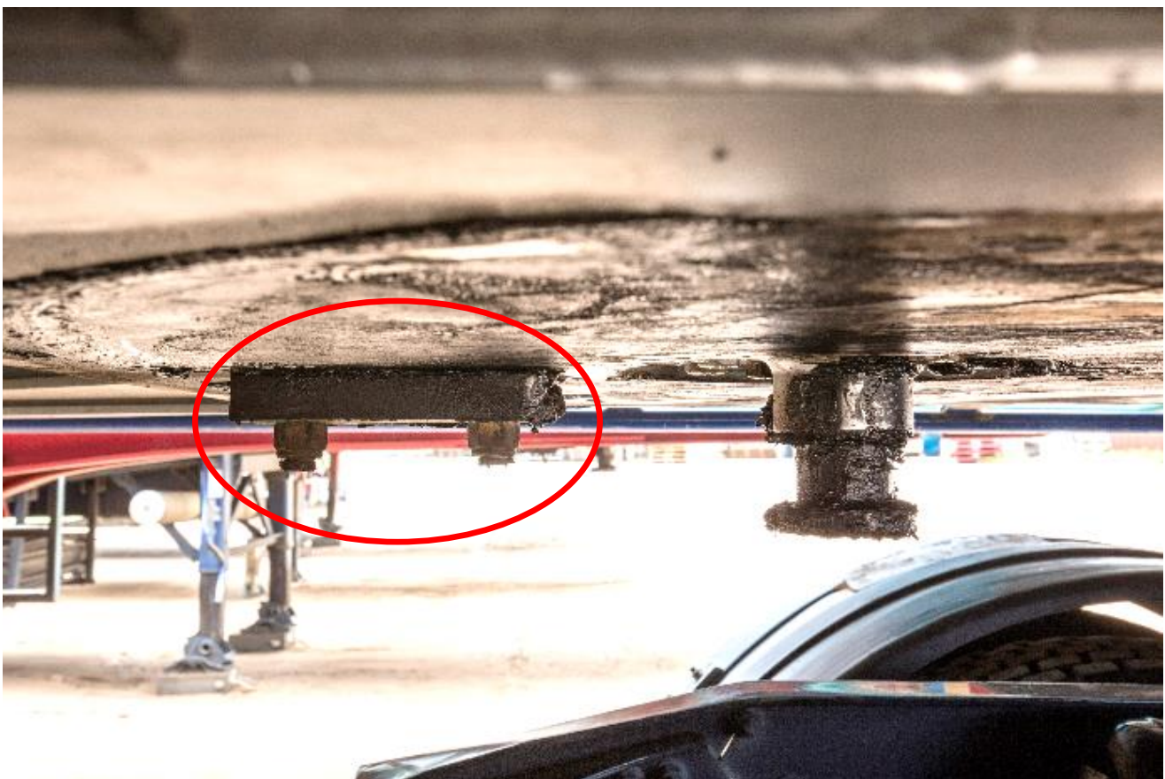
Figure 3: Trailer skid plate locking key (block)
